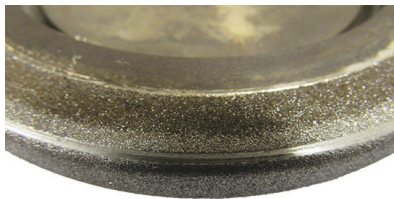
CBN wheel damaged by premature grinding of the tooth tip.
