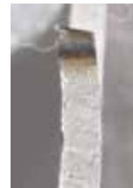
Excessive burning on the tip is a sure sign that the CBN wheel is starting the grind at the tip of the tooth, as opposed to the full "plunge" profile grind.
