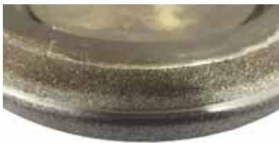
CBN wheel damaged by premature grinding of the tooth tip.
