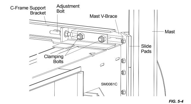
1. Raise the saw head to the top of the vertical mast and secure the saw head with a chain at the top, or shim it underneath. Check the top set of four pads. The outer two pads should be touching the mast rails. There should be a small gap (just wide enough to slide a business card through) between one of the inner pads and the mast rail.
