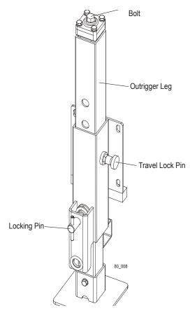
FIG. 2-16. ADJUSTABLE OUTRIGGER.
