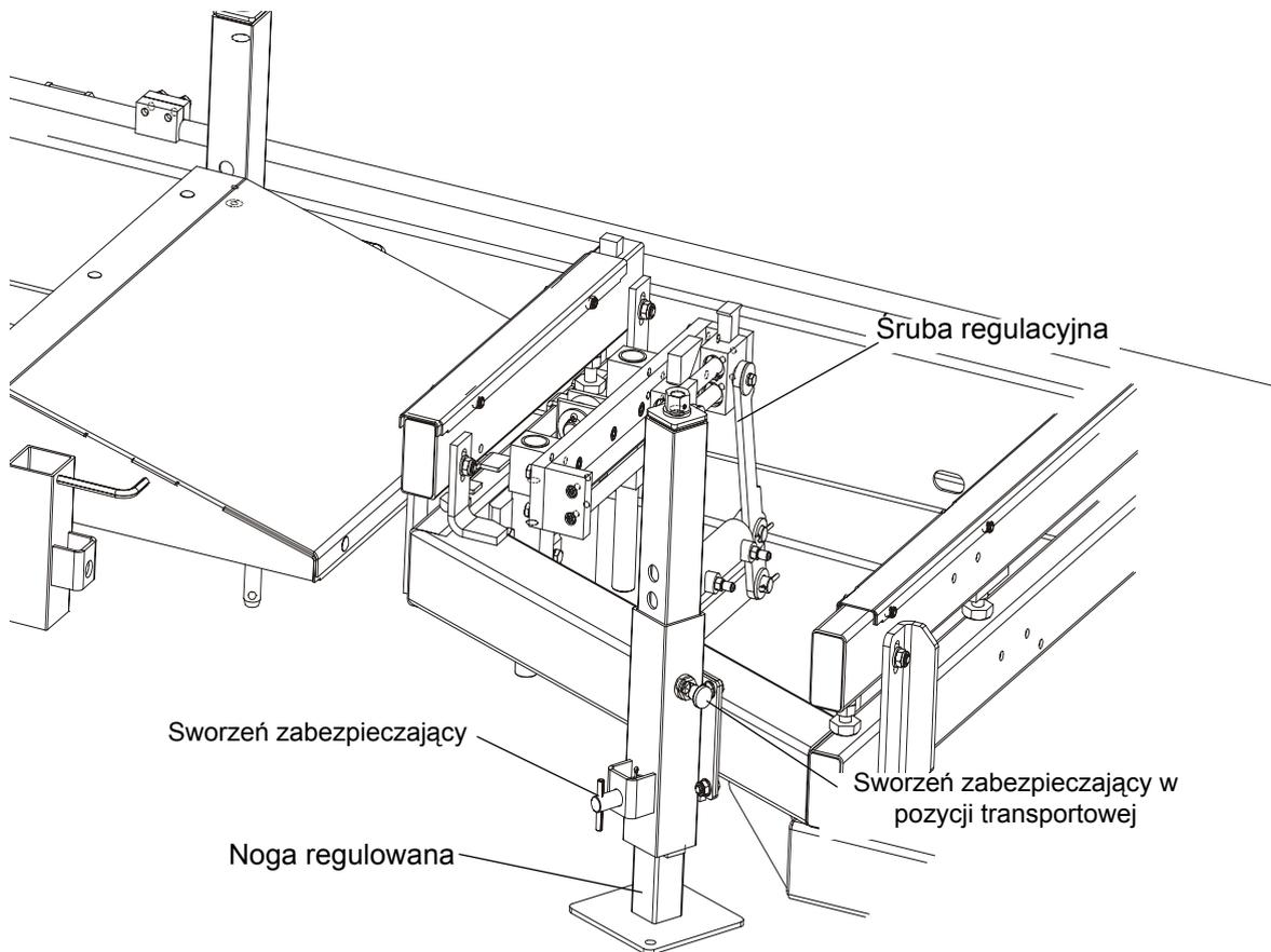
**FIG. 2-3. OUTRIGGER ADJUSTMENT.**
