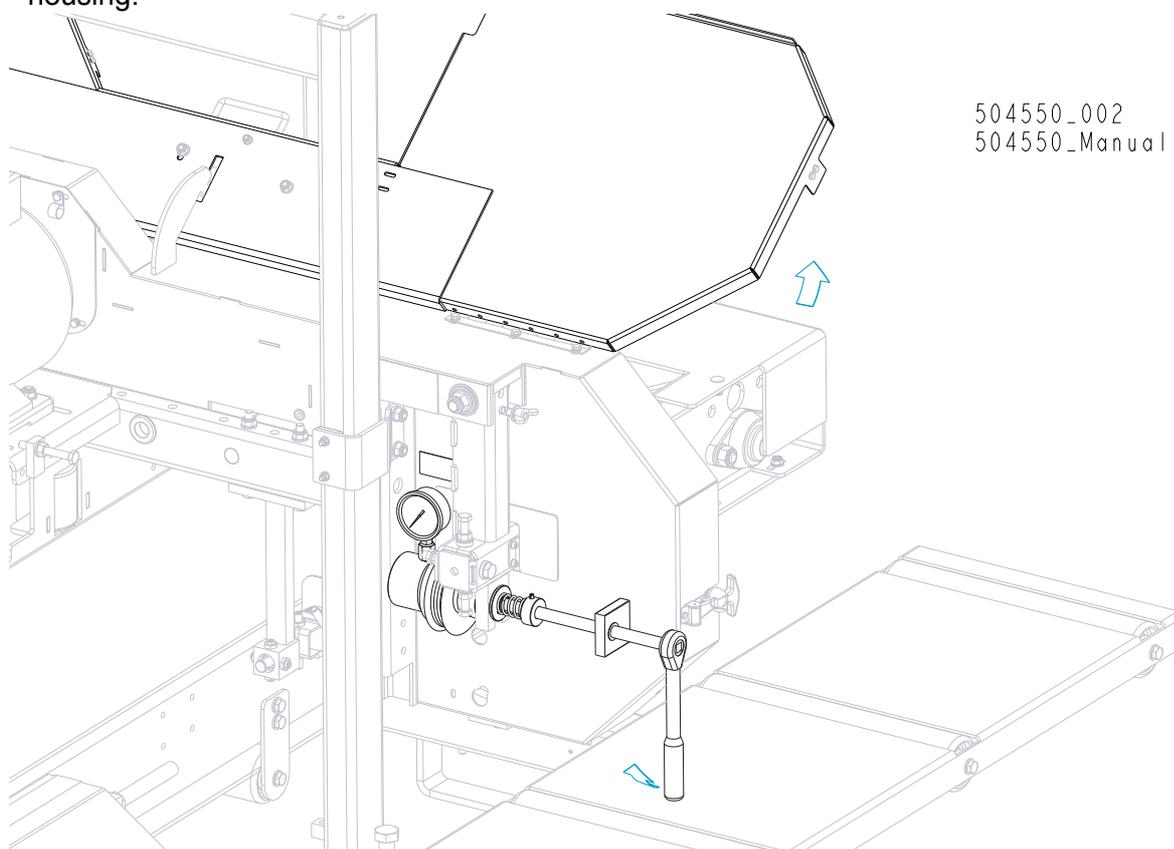
Install a new blade on the blade wheels. When installing the blade, make sure the teeth are pointing the correct direction. The teeth located between the blade guide assemblies should be pointing toward the sawdust chute.
