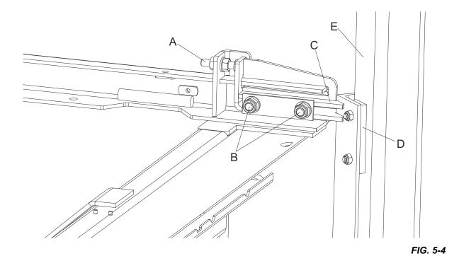
1. Raise the saw head to the top of the vertical mast and secure the saw head with a chain at the top, or shim it underneath. Check the top set of four pads (D). The outer two pads should be touching the mast rails (E). There should be a small gap (about 0,2mm wide) between one of the inner pads and the mast rail.
