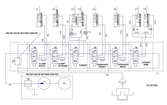
FIG. 1-2 HYDRAULIC SCHEMATIC.
