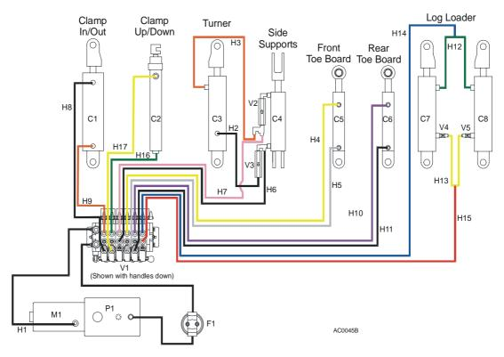
FIG. 1-3 HYDRAULIC LAYOUT DIAGRAM.
