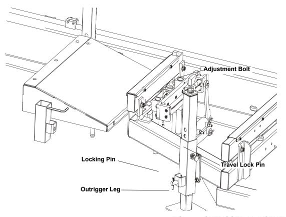
FIG. 2-3. OUTRIGGER ADJUSTMENT.
