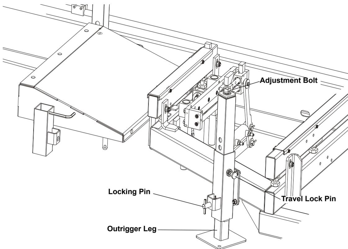
**FIG. 2-3. OUTRIGGER ADJUSTMENT.**
