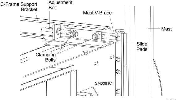
1. Raise the saw head to the top of the vertical mast and secure the saw head with a chain at the top, or shim it underneath. Check the top set of four pads. The outer two pads should be touching the mast rails. There should be a small gap (just wide enough to slide a business card through) between one of the inner pads and the mast rail.
