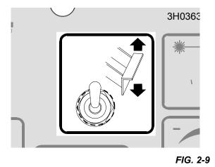
When the blade reaches the end of the log, the arm will drop down to catch the board and drag it back toward the operator as the saw head is returned.
