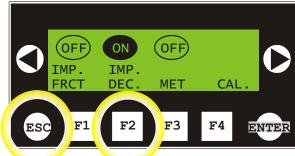
Push "F1" for Imperial Fractions, "F2" for Imperial Decimals or "F3" for Metric units. The unit selected will show "ON" above the button label. Push ESC to return to the main screen.
