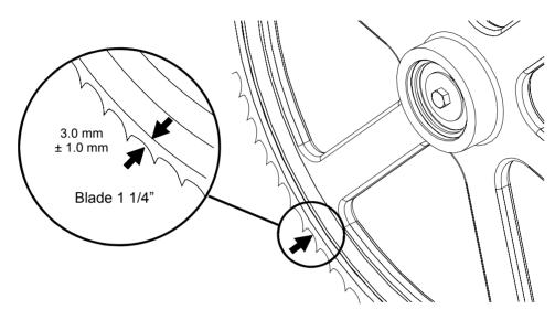
FIG. 6-5 See Figure 6-6. Use the cant control adjustment, shown on the figure below, to adjust the idle-side blade wheel. If the blade is too far forward on the wheel, turn the cant control counter clockwise. If it is too far back on the wheel, turn the cant control clockwise.
