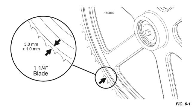
To adjust where the blade travels on the idle-side and drive-side blade wheel, see next section in this manual.
