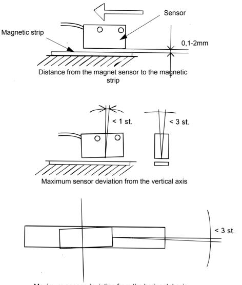
Maximum sensor deviation from the horizontal axis
