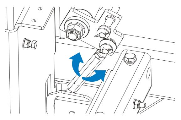
To tighten - turn the bolt clockwise; to loosen - turn it counterclockwise.
