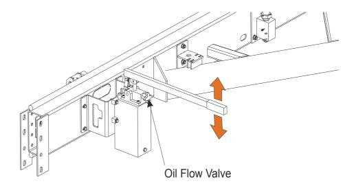
**4.** Lower the loading arms by opening the oil flow valve. To open the valve, turn the valve knob counterclockwise. Leave the loading arm halfway down while positioning the log on the bed. This will prevent the log from rolling of the bed.
