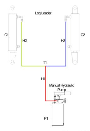
FIG. 1-2 HYDRAULIC LAYOUT DIAGRAM.
