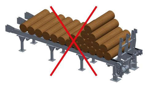
FIG. 2-3 INCORRECT WAY TO LOAD LOGS
