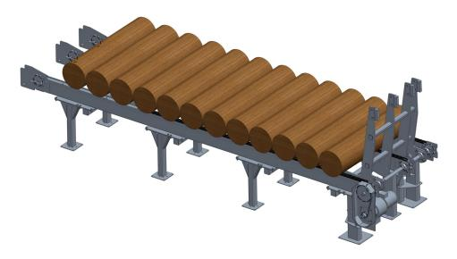
FIG. 2-2 CORRECT WAY TO LOAD LOGS
