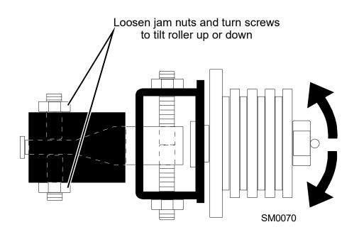
**5.** Measure the distance from the bottom of the tool to the top of the feed track chain at the rear end of the tool. If the measurement does not equal the other two measurements taken, readjust the vertical tilt of the blade guide.
