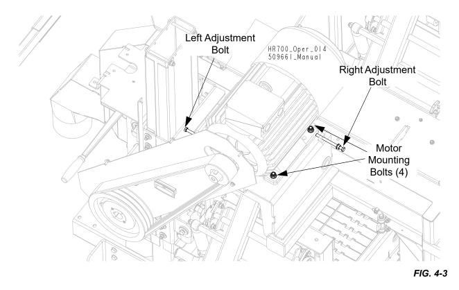
Periodically check the belt for wear. Replace if damaged or worn.
