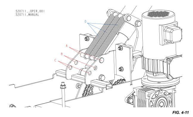
**See Figure 4-12.** To adjust the height of the hold-down arm above the feed track, loosen the nuts (A), use the adjustment bolt (B) and tighten the nuts (A). **NOTE:** The bolts must be adjusted evenly.
