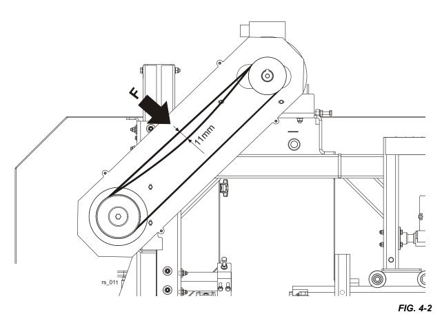
To adjust the drive belt tension:
