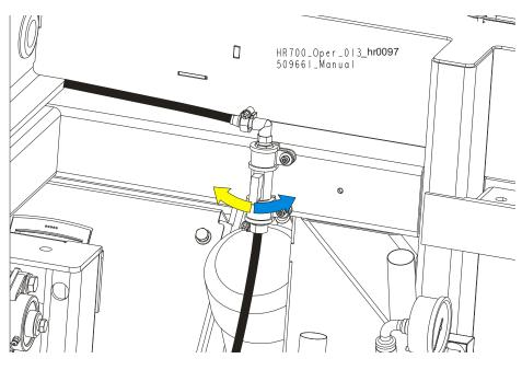
**See Figure 2-22.** Use the manual valve on each saw head to adjust the amount of water flow.
