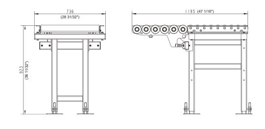
**See Figure 6-4.** See the figure below for the major dimensions of the Cross Roller Table (SLPCRT).
