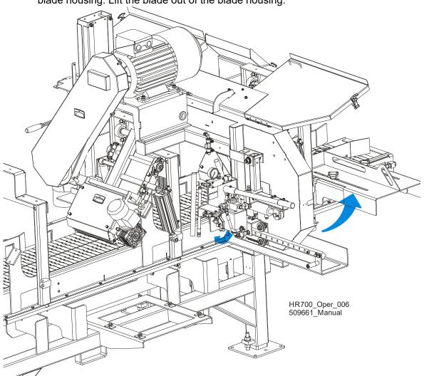
blade housing. Lift the blade out of the blade housing.
