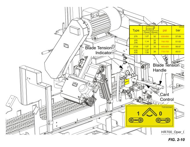
**CAUTION!** Release the blade tension when the resaw is not in use (for example at the end of a shift). Tension the blade again before starting the motor.
