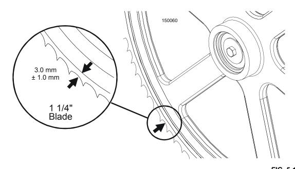
FIG. 5-10 See Figure 5-11. Use the cant control adjustment to adjust the idle-side blade wheel. If the blade is too far forward on the wheel, turn the cant control counterclockwise. If it is too far back on the wheel, turn the cant control clockwise.
