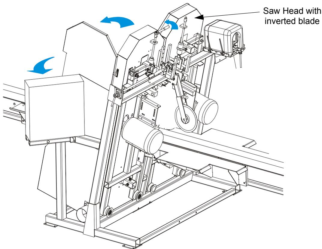
Install a new blade around the two blade wheels so that the teeth located between the blade guide assemblies point to the infeed table. Make sure the teeth are pointing the correct direction.
