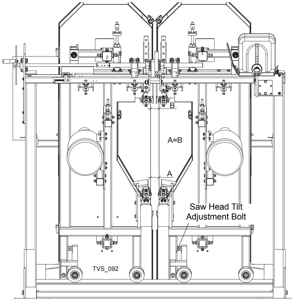
3. Use the square to check if the saw heads are perpendicular to the table. Adjust if necessary.
