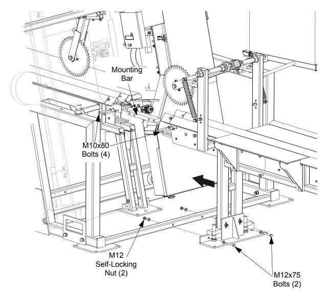
with the TVS frame using the two M12x75 bolts, washers and self-locking nuts.
