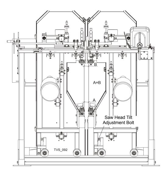
**3.** Use the square to check if the saw heads are perpendicular to the table. Adjust if necessary.
