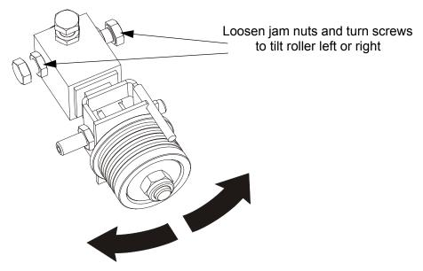
Attach ropes to the lower holes of the alignment bracket. Attach the tools to the blade near the lower blade guide mount blocks and repeat above steps. Adjust the horizontal tilt of this guide if necessary.
