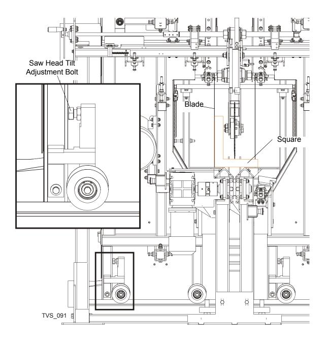
2. Measure distances between the blades at the lowest and the highest points. If the measurements are not the same, adjust the saw heads using the tilt adjustment bolts shown below.
