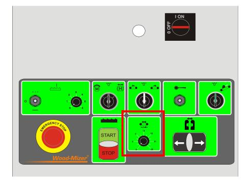
See Figure 2-7. The speed at which the feed track moves is adjustable. The feed track
